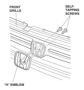
5. Attach the "H" emblem to the new front grille with the two self-tapping screws you removed.
