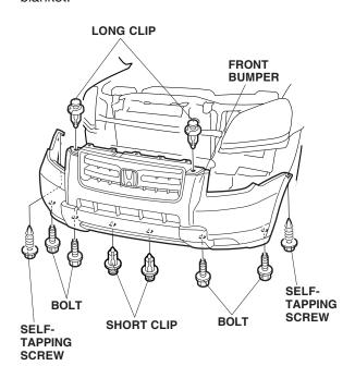
Remove the five clips and five retaining tabs that secure the existing front grille to the front bumper.
