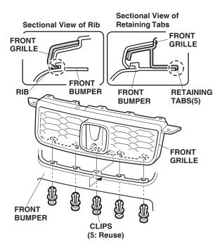
7. Reinstall all removed parts. Check that all clips and retaining tabs are installed securely.
