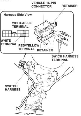
37. Slide the combination light switch onto the steering column and secure the combination light switch with the two screws removed in step 35. Hold the combination light switch case securely against the column while tightening the screws, do not push on the lever.
