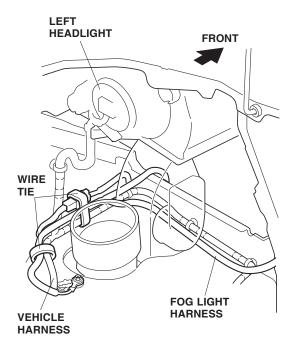
14. At the left front bulkhead panel, secure the fog light harness to the vehicle harness with two wire ties.
