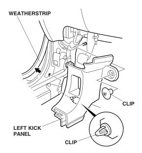
26. Remove the upper clip from the left kick panel, then pull the left kick panel out toward you to release the remaining clip.
