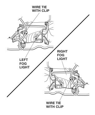
22. On each side attach the fog light harness wire tie with clip to each fog light bracket, then reinstall the front bumper
