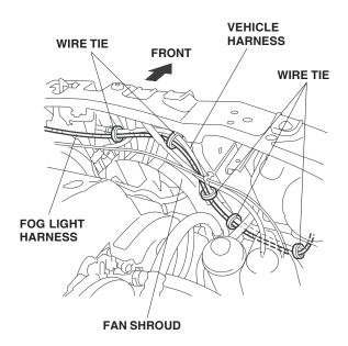
17. Below the right headlight, secure the fog light harness to the vehicle harness with two wire ties.
