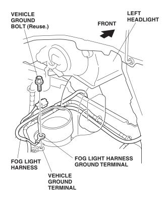
8. Route the short end of the fog light harness 2-pin connector under the left headlight. Locate the 1-pin connector blue-taped to the vehicle harness under the left headlight. Remove the blue tape to free the connector. Plug the vehicle 1-pin connector into the fog light harness 1-pin connector.
