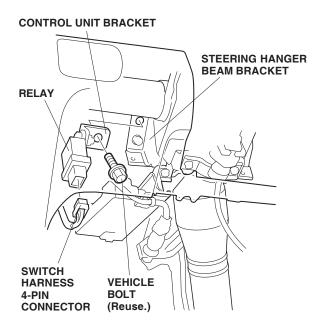
33. Remove the vehicle bolt that secures the steering hanger beam bracket, and attach the control unit bracket with this bolt.
