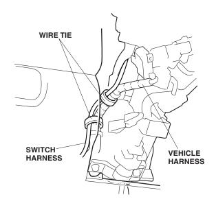
40. Secure the switch harness to the vehicle harness with two additional wire ties in the areas shown.
