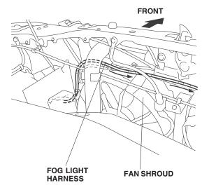
12. Continue routing the fog light harness under the vehicle harness to the right side of the vehicle. Route the harness under the right headlight through the opening near the right horn.
