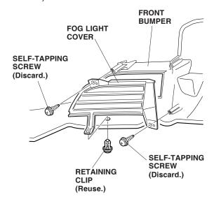
19. Install the left fog light on the front bumper using the retaining clip you removed and three 5 x 16 mm self-tapping screws.
