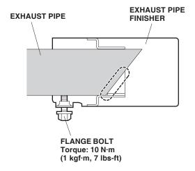
Start the engine and rev it up a few times. Listen for vibration from the exhaust pipe finisher and adjust if necessary.
