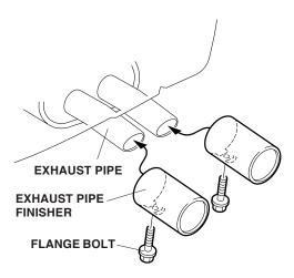
2. With the flange bolts facing down, slide the exhaust pipe finishers onto the exhaust pipes until it bottoms. If necessary, use a rubber mallet to tap the exhaust pipe finishers into place.
