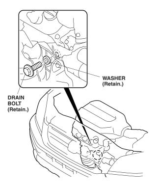
4. While wearing heavy gloves, install the new aluminum washer and the engine block heater into the bolt hole using a 24 mm socket and a torque wrench. Torque the engine block heater to 60 N·m (44 lb-ft).
