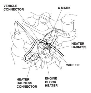
7. Align the remaining B mark on the heater harness with the base of the fan shroud rib and secure the heater harness to the fan shroud with a wire tie.
