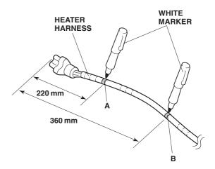
6. Plug the connector end of the heater harness into the engine block heater. Align the A mark you just made on the heater harness with the end of the vehicle connector and secure the heater harness to the vehicle connector with a wire tie.
