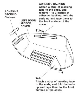
Attach strips of masking tape to the ends of the upper adhesive backing and center tab and remove 1 to 2 inches of the backing. Fold the ends up and tape them temporarily to the surface of the door mirror cover. Remove the remaining adhesive backings.
