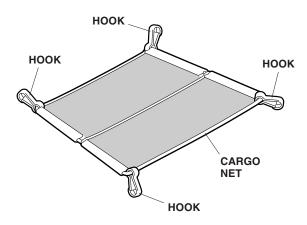
6. Attach the hooks of the cargo net to the front, and to the rear anchors.
