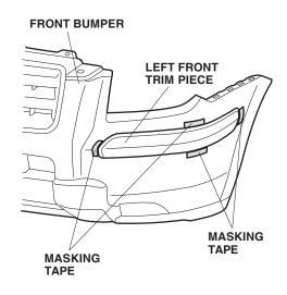
11. Attach a strip of masking tape to the ends of the four adhesive backings shown, and peel back 2 to 3 inches from the ends. Fold the ends up and tape them to the front of the trim piece. Remove the remaining two adhesive backings.
