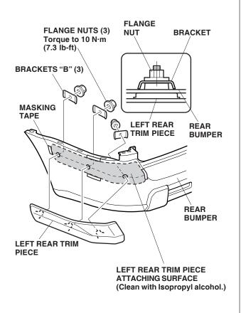
24. Position the left rear trim piece on the rear bumper, and align it with the masking tape. Install one bracket "B" and one flange nut over each stud on the trim piece. Note the direction of the brackets. 25. While holding light pressure on the trim piece, slowly and carefully remove the adhesive backings.
