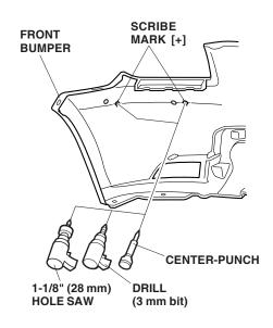
While wearing eye protection, drill an 1-1/8" (28 mm) hole through each of the center-punched marks. First drill with a 3 mm bit, and finish with an 1-1/8" (28 mm) hole saw. Remove any burrs from the edges of the holes.
