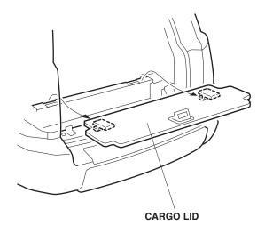
2. Turn the lid over, and locate the eight marks on the surface of the cargo lid.
