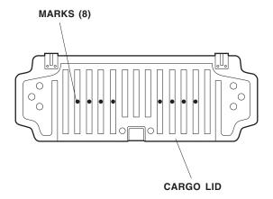
3. While wearing eye protection, drill a 3 mm pilot hole and finish with a 10 mm hole through one set of two marks as indicated, depending on which side you want to mount the bicycle attachment. Drill the appropriate holes depending on the type of bicycle to be carried.
