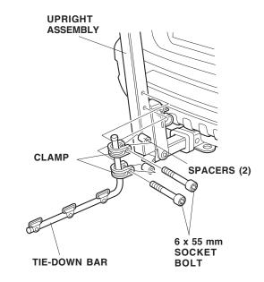
6. Turn the tie-down bar 90° in the direction shown. This is the stored position.
