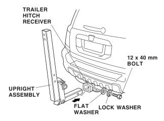
2. Lower the bicycle arm bracket onto the upright assembly as shown.
