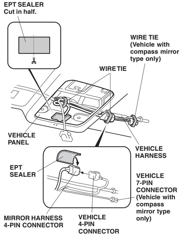
22. Cut the EPT sealer into exact halves. Wind one of the two halves of the EPT sealer you just cut onto the mirror harness 4-pin connector.
