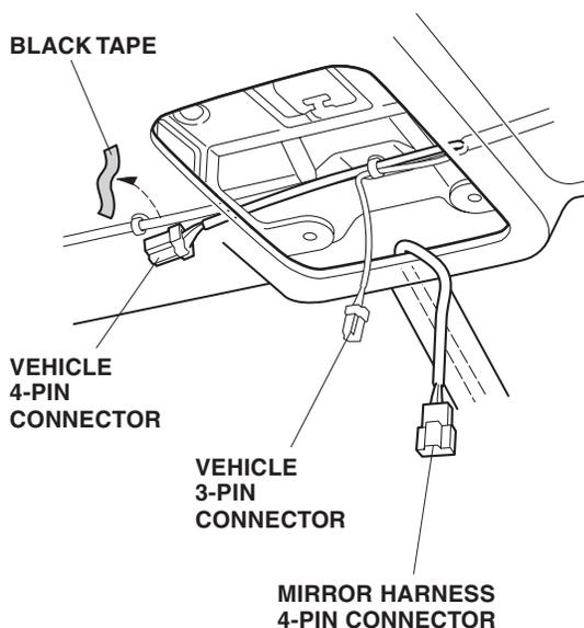
16. Plug the mirror harness 4-pin connector into the vehicle 4-pin connector.
