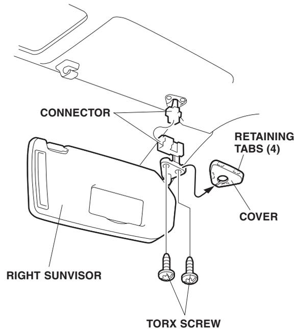
7. Remove the right sunvisor (two Torx screws and unplug the connector).
