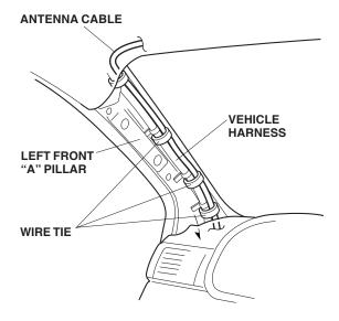
Route the antenna cable along the vehicle harness toward the driver's under-dash fuse box. Secure the antenna cable with one wire tie in the area shown.
