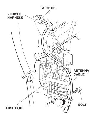
20. Remove the bottom bolt from the driver's underdash fuse box. 21. Turn up the carpet. Route the antenna cable under the carpet and next to the vehicle harness.
