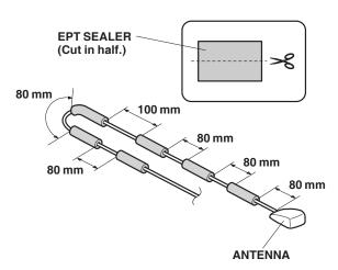
15. Using the isopropyl alcohol, clean the areas where the antenna will attach. Remove the adhesive backing from the antenna, and attach the antenna to the front window at the locations shown. Install the antenna by applying sufficient pressure.
