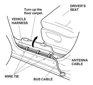
28. Continue routing the BUS cable underneath the driver seat.
