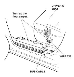
29. Secure the antenna cable and bus cable to the vehicle harness at the carpet opening with one wire tie.
