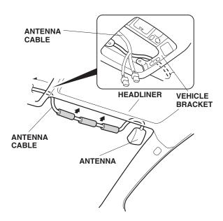
17. Embed the antenna cable in the headliner, and secure it with one wire tie to the vehicle harness.
