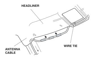
18. Route the antenna cable along the left front "A" pillar. Secure the antenna cable to the vehicle harness with four wire ties.
