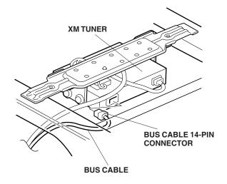
40. Fold the excess length of antenna cable and bus cable, then secure the folded cables to the vehicle pipe with two wire ties.
