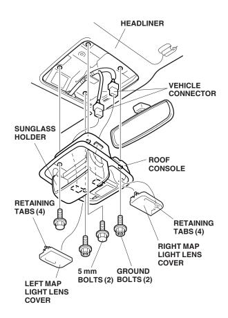
Disconnect the two vehicle connectors, and remove the roof console. 5. Remove the cover from the left sunvisor.
