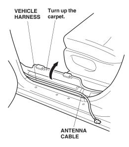
22. Turn up the carpet. Continue routing the antenna cable underneath the driver's seat and out through the flap in the carpet.
