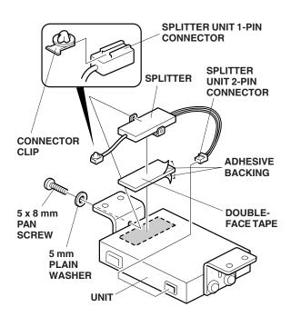
32. Remove the adhesive backing from the other side of the double-sided tape, then install the splitter to the XM tuner with one 5 x 8 mm pan screw and one 5 mm plain washer.
