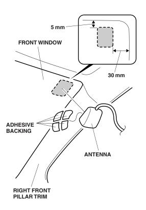
16. Route the antenna cable so that it routes inside the headliner.
