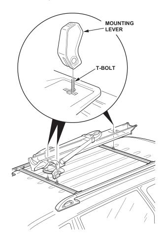
9. Position the bike attachment on the front and rear crossbars. Turn and adjust the mounting lever to lock the bike attachment to the roof rack. Check for firm pressure while you push down on the mounting lever to lock it into place.
