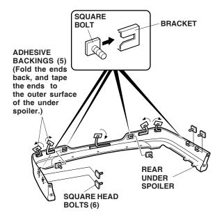
Attach a strip of masking tape to the end of each adhesive backing, then pull back 1½ to 2 inches of adhesive backing. Fold the ends back, and tape them to the outer surface of the spoiler with masking tape. 7. Using isopropyl alcohol on a shop towel, clean the rear spoiler areas where the adhesive collars will attach. Remove the adhesive backing from each adhesive collar, and attach the collar to the inside of the rear spoiler in the areas shown.
