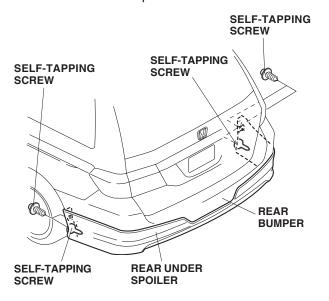
14. Install the self-tapping screws at the fenderwell.
