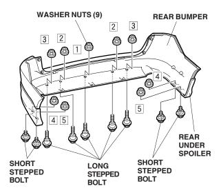
12. While holding light pressure on the under spoiler, carefully remove the adhesive backings from the under spoiler. After attaching, hold the under spoiler firmly against the rear bumper with the palm of your hand for 30 seconds, particularly at the edges.
