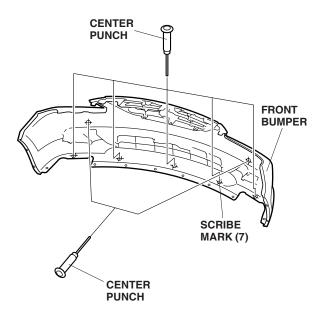
5. While wearing eye protection, drill two 8 mm holes through the front bumper. First drill with a 3 mm drill bit, then finish with an 8 mm drill bit.
