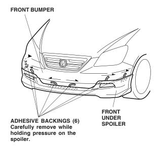
17. While holding the edge of the spoiler against the bumper, tighten the four self-tapping screws installed in step 14.
