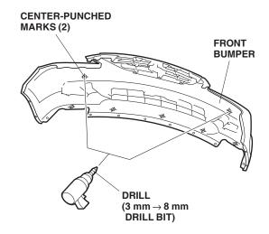
6. While wearing eye protection, drill five 10 mm holes through the five center-punched marks along the bottom of the bumper. First drill with a 3 mm drill bit, then with a 6 mm drill bit, and finish with a 10 mm drill bit.
