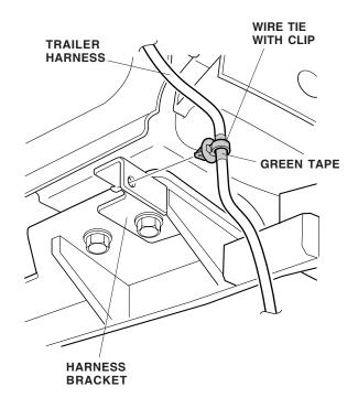
Secure the trailer harness to the trailer hitch with four wire ties.
