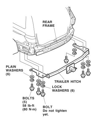
9. Torque the five trailer hitch bolts to 58 lb-ft (80 N·m).
