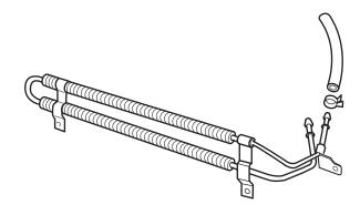
43. Locate and remove the old power steering cooler clip. Discard the clip.
