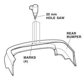
7. Using a utility knife, cut along the marked area, and remove the center section of the bumper. Using a file, remove any burrs from the bumper.
