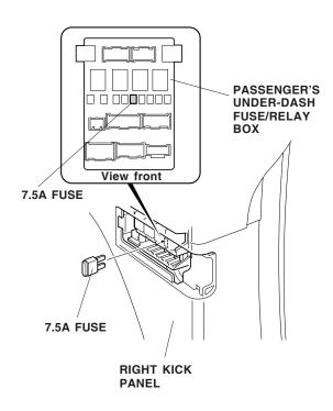
34. Attach the fuse label (7.5A) to the fuse cover as shown.
