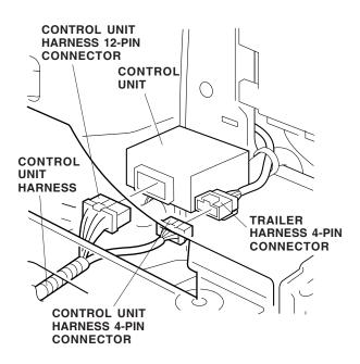
26. Attach the 7.5A fuse label to the fuse case on the control unit harness.
