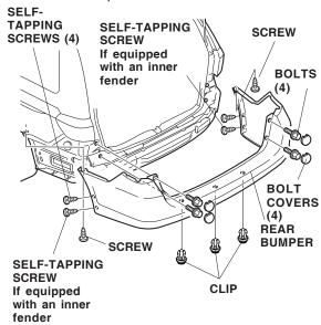
4. On the inside of the rear bumper, place the template on the bumper with the hole in the template over the center clip hole.
