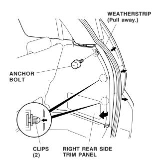
With an assistant gently pulling out on the right rear side trim panel, plug the control unit harness 8-pin connector into the rear junction box. Secure the control unit harness to the vehicle harness with two wire ties.
