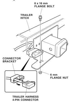
20. Secure the trailer harness to the trailer hitch with two wire ties.
