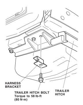
17. Attach one wire tie with clip to the trailer harness at the green tape, then insert the clip into the hole in the harness bracket.
