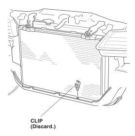
44. Position the ATF cooler on the front bulkhead, and align the bolt holes in the cooler with the threaded holes in the bulkhead. Install the three 6 x 12 mm bolts (supplied) into the threaded holes to secure the ATF cooler.
