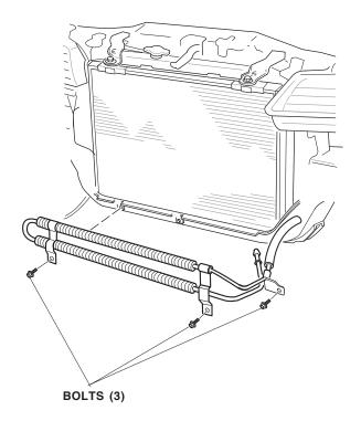
45. Remove the ATF return line from the radiator return pipe, and attach it to the lower ATF cooler pipe using one new hose clamp from the kit.
