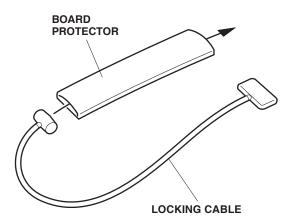
14. Insert the locking cable plate into the slit of the snowboard carrier. To carry one snowboard, insert the plate into the lowest slit. To carry two snowboards, use one of the upper three slits in the carrier.
