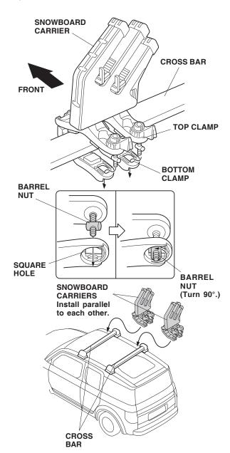
8. Turn the knobs on the top clamp to tighten the front carrier.
