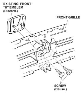
4. Align the two pins on the front gold "H" emblem with the holes in the front grille and secure the emblem with the two screws you just removed.
