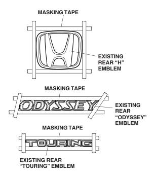
7. Remove the "H", "ODYSSEY" and "TOURING" emblems from the body by cutting the outer edges with a piece of string.
