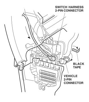
75. At the fuse box, secure the switch harness to the vehicle harness with three wire ties.
