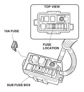
**LX Model:** Install the 10A fuse into the underhood fuse/relay box in the location shown.
