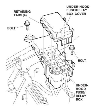
18. Remove the under-hood fuse/relay box cover (four retaining tabs).
