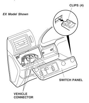
67. Remove the switch lid (two retaining tabs).
