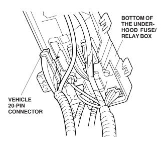
29. Get the short subharness. Plug the 1-pin terminal from the short subharness into the back of the vehicle 20-pin connector.
