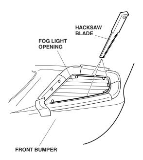
On the inside of the front bumper, cut out the fog light opening from the front bumper using a hacksaw blade. Remove any burrs, and remove the masking tape.
