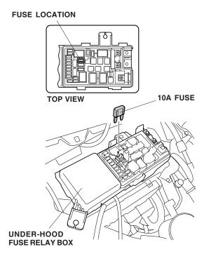
77. **LX Model Only**: Attach the 10A fuse label to the inside of the under-hood fuse relay box.
