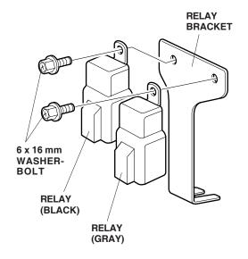
61. Plug the blue fog light harness 4-pin connector into the gray relay. Plug the brown fog light harness 4-pin connector into the black relay.
