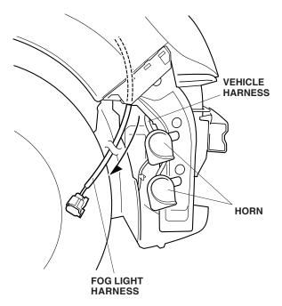
42. Attach the two wire ties with clips on the fog light harness into the holes in the vehicle body.
