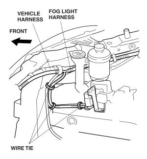
64. With the help of an assistant, plug the fog light harness 2-pin connectors into the fog light connectors, and reinstall the front bumper in its original position. Be careful that the fog light harness does not get caught between the bumper and the splash shield.
