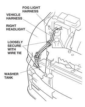
41. Route the right fog light harness 2-pin connector along the vehicle harness and into the bumper area.
