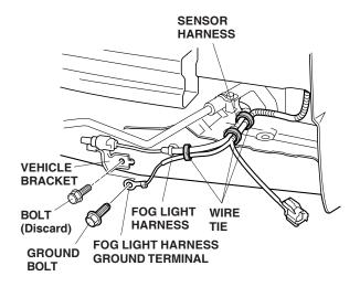
55. **EX model with AUTO air:** Remove the bolt from the vehicle bracket. Secure the ground terminal from the fog light harness to the vehicle bracket using the ground bolt supplied.
