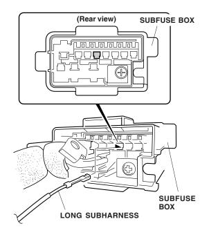
25. Secure the long subharness to the subfuse box harness with one small wire tie.
