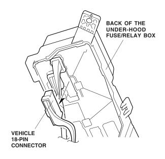
32. Get the fog light harness. Plug the 1-pin white/ green and the 1-pin red/green terminals into the back of the 18-pin connector in the locations shown.
