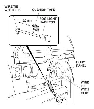
52. Attach the wire tie with clip on the fog light harness into the hole in the body panel.
