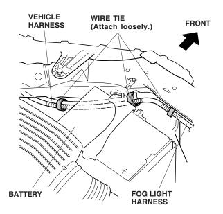
51. Locate the wire tie with clip near the end of the fog light harness. Wrap a cushion tape around the fog light harness at the measurement shown.
