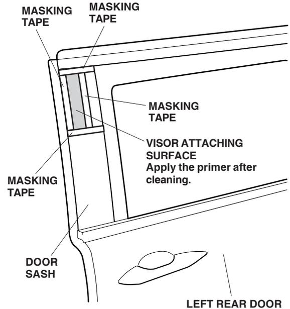
9. On the back of the left rear door visor, peel back 1 to 1 1/2 inches (26 to 38 mm) of the adhesive backing, and tape the backing to the front surface of the left rear door visor.
