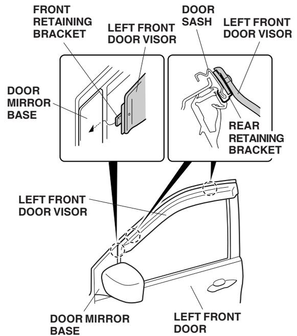
6. While holding light pressure on the door visor, carefully remove the adhesive backings.
