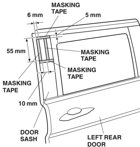
8. Apply primer to the cleaned surface. Remove the masking tape.
