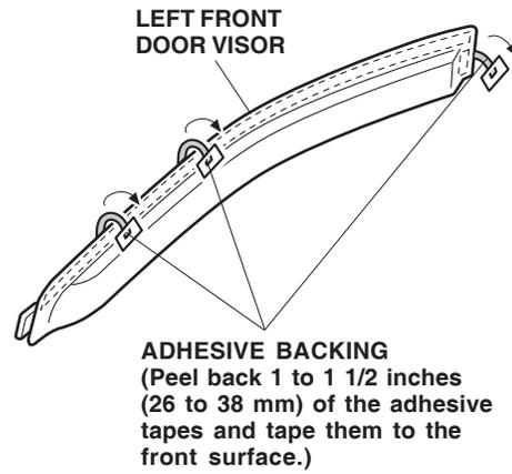
5. Position the left front door visor on the door. Push the front retaining bracket into the door mirror base; push the two rear retaining brackets into the door sash.
