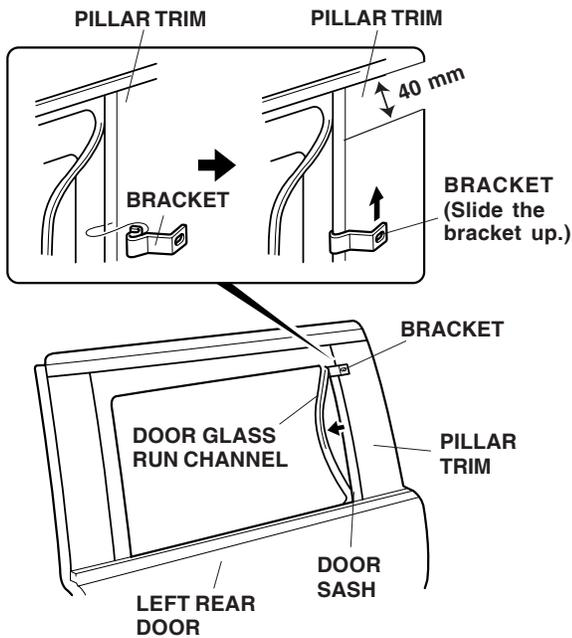
11. Position the left rear door visor on the door sash. Push the two retaining brackets into the door sash.
