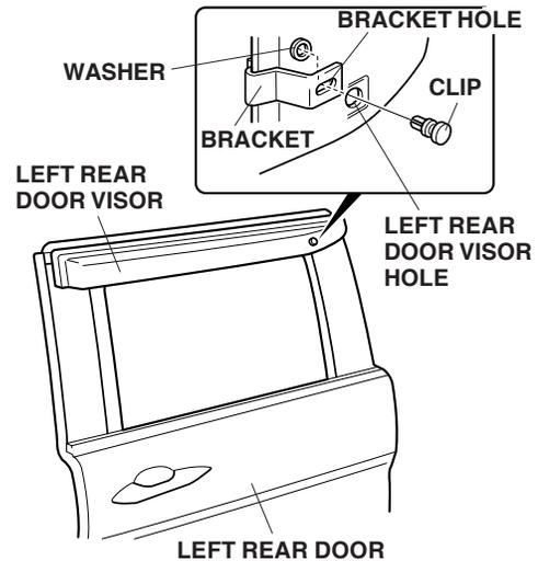
14. While applying light pressure on the left rear door visor, carefully remove the adhesive backings.
