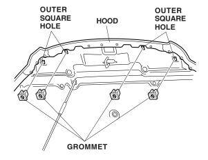
Push a plastic grommet into each of the four outer square holes in the hood.
