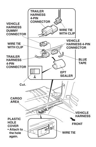
10. Secure the trailer harness to the vehicle harness with one wire tie as shown. Route the trailer harness through the square hole in the inner panel, and reattach the plastic hole cover. 11. Route the trailer harness down through the clearance between the rear bumper beam and body panel, and reinstall the rear bumper.
