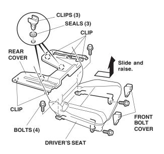
13. Remove the two front bolt covers, then remove the four bolts that fasten the driver's seat side rails so that the driver's seat can be lifted. 14. Remove the driver's door side sill trim (nine clips and two retaining tabs). Take care not to damage the clips and retaining tabs. Be sure to reattach any seals that came off the clips.
