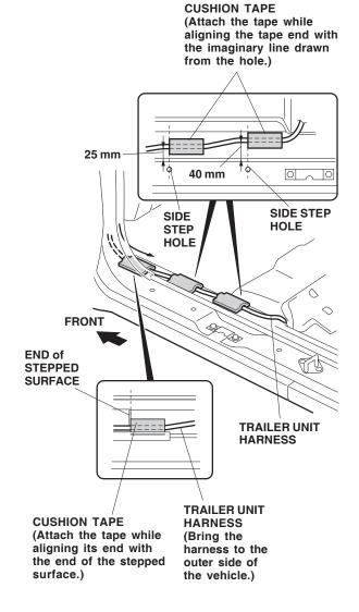
27. Bring the trailer harness to the outer side of the vehicle. Secure the trailer harness with the cushion tape while aligning the end of the tape with the end of the stepped surface of the side step as shown. Clean the surface where the cushion tape will be attached with isopropyl alcohol.
