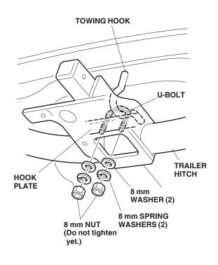
34. Torque all bolts and nuts to their specified torques in the order of 1, 2, and 3.
