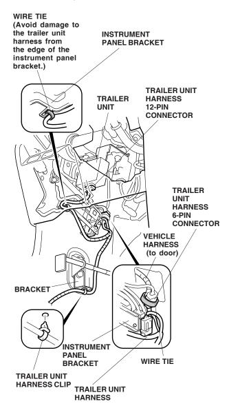
23. Insert the trailer unit harness clip into the hole in the bracket. Secure the 6-pin connector connected in step 19 to the vehicle harness with one wire tie.
