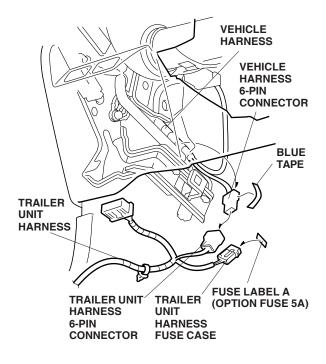
20. Install the fuse case of the trailer unit harness by sliding it onto the coupler holder of the vehicle harness.
