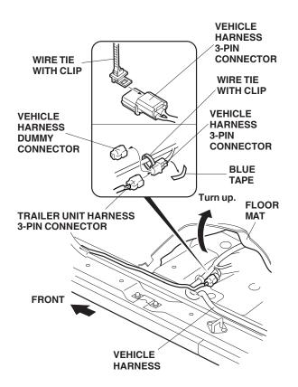
25. Connect the 3-pin connector of the trailer unit harness to the vehicle 3-pin connector. Then secure the trailer unit harness to the vehicle harness with the wire tie with clip installed in step 23.
