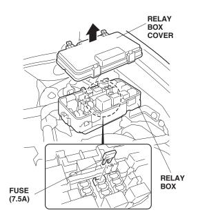
28. Attach the fuse label B (7.5A) over the No.15 on the back of the relay box cover. Reinstall the relay box cover.
