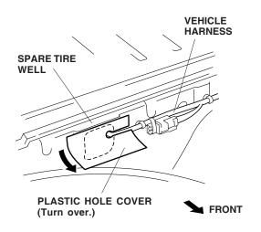
7. Remove and discard the rear left grommet from the body. Attach a piece of steel wire to the trailer harness 4-pin connector, and pull the 4-pin connector through the vehicle grommet hole and into the hole in the spare tire well. Seat the trailer harness grommet in the vehicle grommet hole with the end facing down.
