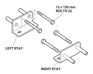
30. From the inboard side of the vehicle frame, slide the right and left stays into the right and left rear frame rails.
