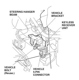
• Combine the vehicle bracket and the unit bracket and attach them with the vehicle bolt you removed. Reconnect the 5-pin connector to the keyless receiver unit.
