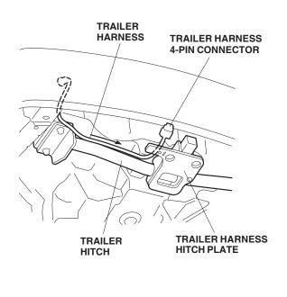
37. Install the connector bracket onto the trailer harness 4-pin connector, and secure them to the trailer hitch with the flange bolt and flange nut.
