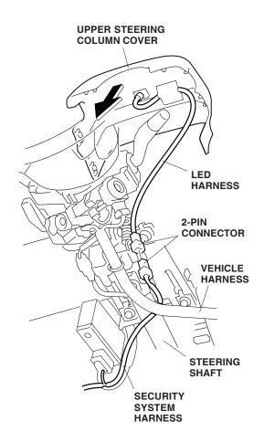
27. Route the security system harness 2-pin connector under the steering shaft, and connect it to the LED harness 2-pin connector.
