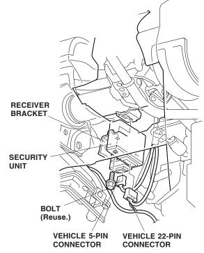
25. Reconnect the vehicle 5-pin connector to the keyless unit.
