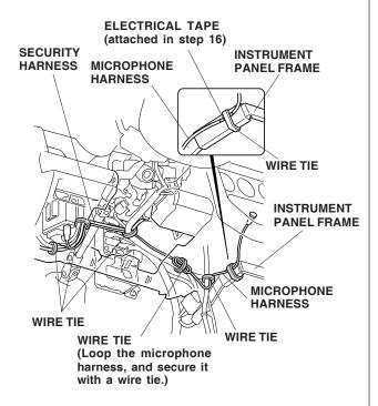
34. Attach the security harness and microphone harness to the vehicle harness with five wire ties in the areas shown.
