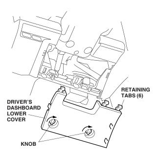
4. Lower the steering wheel using the tilt lever. Remove the two self-tapping screws and one washer-screw from the lower steering column cover. Separate the upper steering column cover from the lower steering column cover by gently pressing down on the six retaining tabs, and release them.
