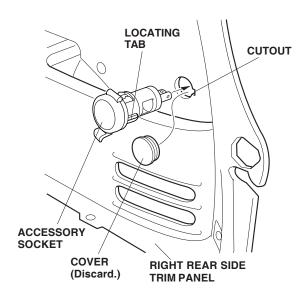
16. Behind the right rear side panel, locate the 2-pin connector blue-taped to the vehicle harness. Remove the blue tape to free the 2-pin connector, then plug the 2-pin connector into the accessory socket.
