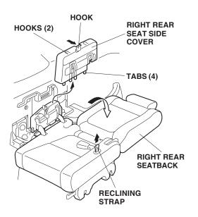
7. Unlock the right rear seat by pulling the right rear seat foot lock release strap out toward you.
