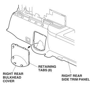
14. Remove the rear portion of the right rear side trim panel by pulling it out toward you (three clips and three retaining tabs). It is not necessary to remove the entire trim panel.
