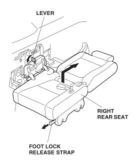
8. Push the lever in the direction shown, then remove the right rear seat by lifting the rear of the seat and sliding the seat through the rear of the vehicle.
