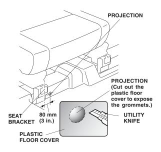
2. Install an anchor to each of the three grommets using one self-tapping screw for each anchor.
