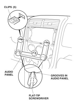
4. Remove the four self-tapping screws that fasten the audio unit, and pull the unit out toward you. Unplug the vehicle connector and the antenna lead from the back of the AM/FM CD tuner, and remove the audio unit from the instrument panel.
