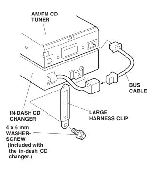
Secure the BUS cable connectors to the indash CD changer with the large harness clip. Get the EPT sealer from the attachment kit. Wrap the EPT sealer around the screw head in the area shown.
