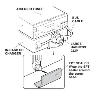
8. Plug in the vehicle connector and the antenna lead in to back of the AM/FM CD tuner, then reinstall the audio unit using four screws.
