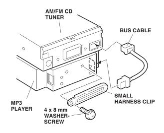
• Secure the BUS cable with the small harness clip.
