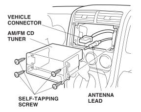
5. Remove the four washer-screws and two selftapping screws that fasten the right and left brackets to the AM/FM CD tuner and pocket. Save the pocket, screws, and brackets for your customer.
