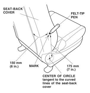
6. Using a utility knife, make two 70 mm (3 in.) cuts in the seat-back cover. Using these 70 mm (3 in.) cuts as a guide, cut out the seat urethane to expose the seat base.
