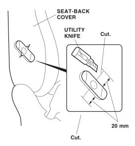
5. Using a felt-tip pen and tape measure, measure and mark the seat-back cover as shown. Push in on the mark, and confirm that the mark is centered over the hole in the seat base.
