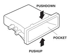
4. Position the audio unit on the pocket and install the two brackets with the four 5 x 8 mm washerbolts and two 4 x 12 mm self-tapping screws.
