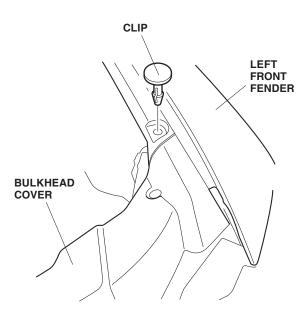
Install one new clip with a snap-screw(B) into the hole where you removed the clip, and tighten the snap-screw(B).
