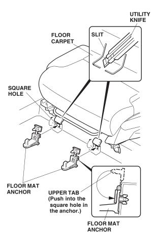
Push the lower tab of the anchor into the square hole concealed under the floor carpet. Pull the upper tab down and push it into the square hole in the anchor as shown. Repeat on the remaining anchor.
