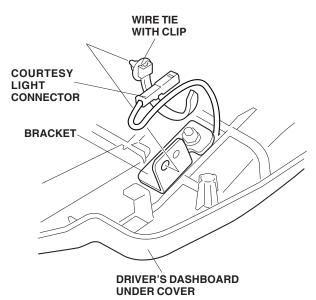
33. Reinstall the insulator to the driver's dashboard under cover, and pass the courtesy light connector through the slit.
