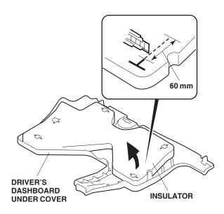
27. Secure the template (A) to the driver's dashboard under cover with tape by aligning it with the square hole at the end of the curve as shown.
