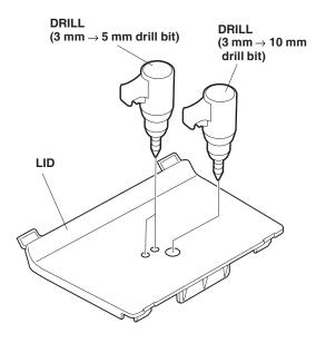
37. Route the courtesy light (with blue tape) connector through the 10 mm hole. Install the courtesy light on the lid with the screw and flange nut.
