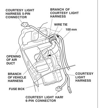
12. Measure the vehicle harness from the point of branch as shown. Secure the courtesy light harness (6-pin connector side) to the vehicle harness with one wire tie.
