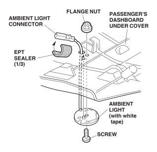
43. Wrap another piece of the EPT sealer that you cut into three equal pieces around the courtesy light connector.
