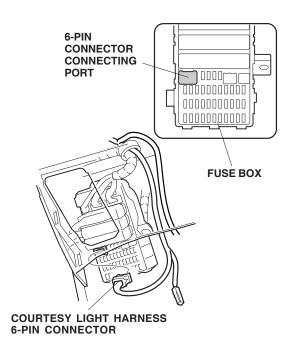
NOTE: If another accessory is already plugged into the 6-pin connector, remove the dummy connector from the other accessory harness, and plug the courtesy light harness into that connector.
