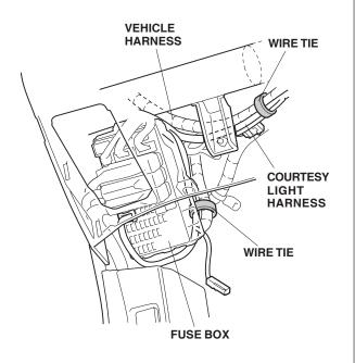
23. Secure the courtesy light harness to the vehicle harness with three wire ties.
