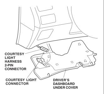
56. Plug the courtesy light harness 2-pin connector to the courtesy light connector on the lid of the dashboard center lower cover, and reinstall the lid.
