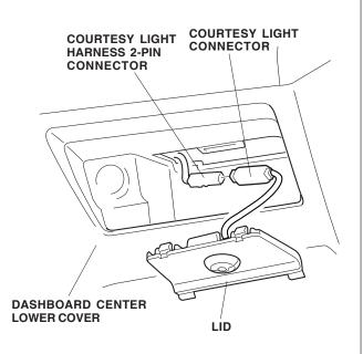
57. Plug the courtesy light harness 2-pin connector to the courtesy light connector on the passenger's dashboard under cover, and reinstall the under cover.
