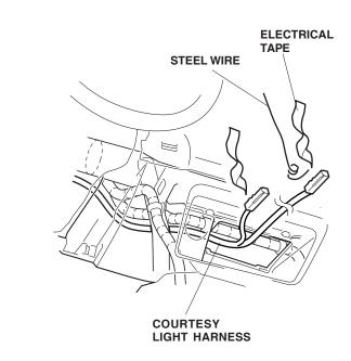
20. Remove the wire and electrical tape from the courtesy light harness.
