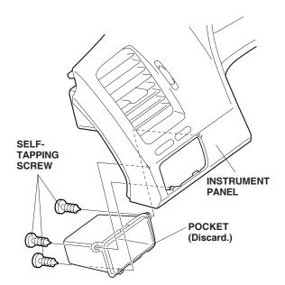
49. Install the switch trim to the instrument panel with the three self-tapping screws.
