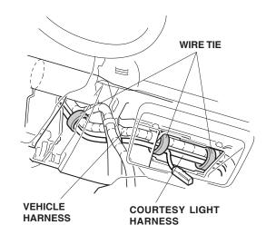
24. Secure the courtesy light harness to the vehicle harness using four wire ties if the vehicle is equipped with the driver's dashboard under cover. Use three wire ties if the vehicle is without the driver's dashboard under cover.
