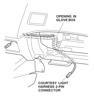
22. Secure the courtesy light harness to the vehicle harness with two wire ties.
