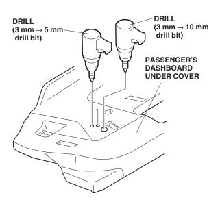
42. Route the courtesy light (with white tape) connector through the 10 mm hole. Install the courtesy light on the passenger's dashboard under cover with the screw and flange nut.
