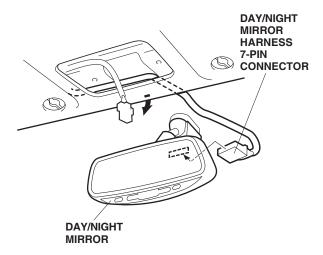
25. Measure the day/night mirror harness in the area shown. Route the day/night mirror harness through the grooves in the upper and lower covers. Attach the lower cover to the mirror stay.
