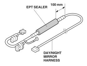
20. Tape a piece of steel wire to the 7-pin connector end of the day/night mirror harness. Pull the 7-pin connector up and out through the clearance between the left front pillar and the instrument panel.
