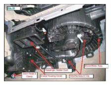
8. Remove the blower motor assembly:
