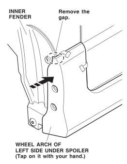
28. Loosely install the front self-tapping screws in the holes on the wheel arch of the left side under spoiler.
