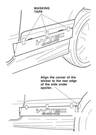
38. Peel back the end of the backing, and spray a natural detergent solution onto the adhesive side.
