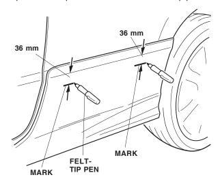
37. Using isopropyl alcohol on a shop towel, attach the sticker to the side under spoiler at the marks you made in step 36. Align the corner of the sticker to the rear edge of the side under spoiler.
