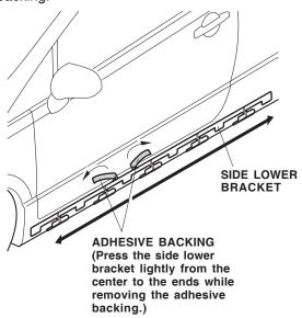
When the workshop room temperature is below 60°F (15°C), warm up the entire side lower bracket to 60°F (15°C) or above before attaching it to the vehicle body.
