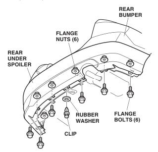
14. While applying pressure on the rear under spoiler, carefully remove the adhesive backings in the sequence shown. After removing, hold the rear under spoiler firmly against the rear bumper with the palm of your hand for 30 seconds.
