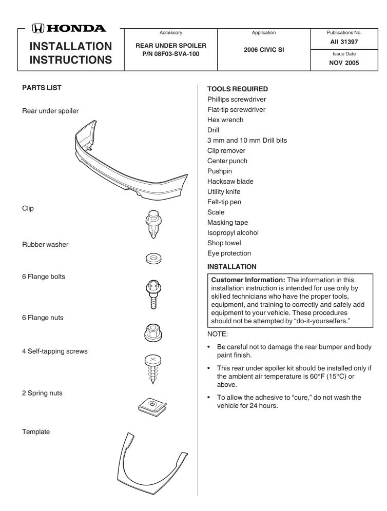
1. Attach the template to the arched section of the rear bumper. Secure the template with strips of tape.
