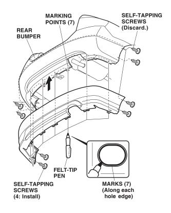
10. While holding pressure on the rear under spoiler, use a felt-tip pen to mark the rear bumper along each hole edge in the bracket on the rear under spoiler.
