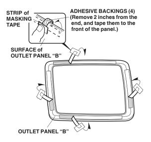
10. Position the outlet panels "A" and "B" on the existing outlet panels. While holding pressure on the outlet panels, carefully remove the adhesive backings from the outlet panels. Press the outlet panels "A" and "B" firmly against the existing outlet panels with the palm of your hand, particularly at the edges.
