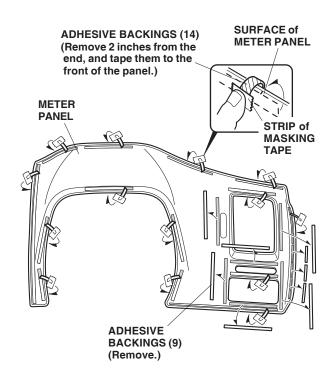
3. Position the meter panel on the existing meter panel. While holding pressure on the meter panel, carefully remove the adhesive backings from the meter panel. Press the meter panel firmly against the existing meter panel with the palm of your hand, particularly at the edges.
