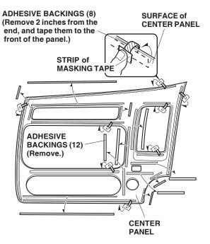
5. Attach a strip of masking tape to the end of each shaded adhesive backing. Peel back 2 in. (5-6 cm) of the adhesive backings, and fold them over as shown. Temporarily attach the strips of masking tape to the outside of the center panel. Remove all remaining adhesive backings from the center panel.
