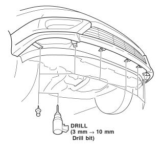
8. Secure the front under spoiler to the front bumper with seven flange-nuts and seven flange bolts.
