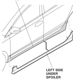
2. Using a tape measure and felt-tip pen, measure and mark the body area shown.
