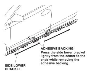
When the workshop room temperature is below 60°F(15°C), warm up the entire side lower bracket to 60°F(15°C) or above before attaching it to the vehicle body.
