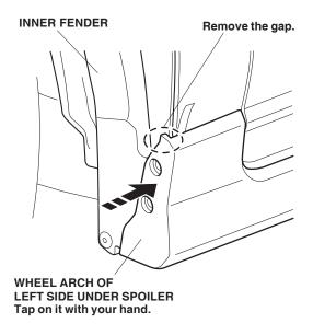
Loosely install the front self-tapping screws in the holes in the wheel arch of the left side under spoiler.
