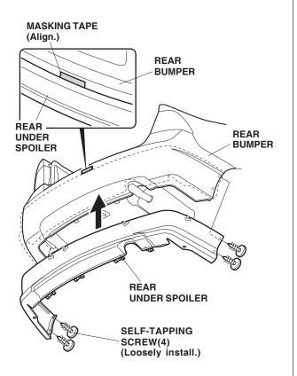
8. While applying pressure to the rear under spoiler, use a felt-tip pen to mark the rear bumper along each hole in the bracket on the rear under spoiler.
