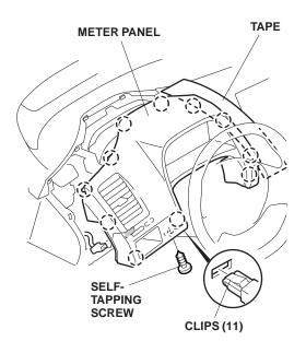
8. Attach the making tape as shown. Remove the center panel (two bolts, ten retaining clips, and unplug the vehicle connectors).
