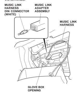
21. Secure the Music Link adapter assembly to the vehicle pipe with two long wire ties.
