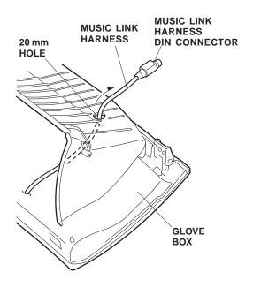
17. Cut the grommet as shown. Attach the grommet to the Music Link harness, and seat the grommet into the 20 mm hole.
