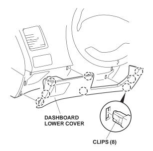
5. Remove the passenger's dashboard lower cover (four clips and two pins).
