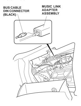
24. Bundle up the excess bus cable, and secure it to the vehicle harness with three wire ties as shown (two wire ties temporarily secured in step 22).
