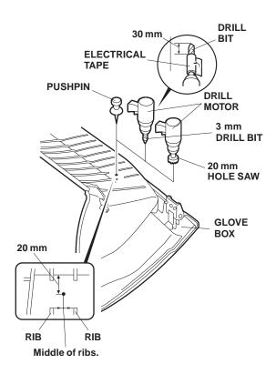
16. Route the Music Link harness DIN connector into the 20 mm hole in the direction shown.
