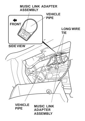
22. Bundle up the excess Music Link harness, and temporarily secure it to the vehicle harness with two wire ties. (Align the mark you made in step 12 with the wire tie as shown.)
