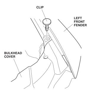
3. Install one new clip with a snap-screw (B) into the hole where you removed the clip, and tighten the snap-screw (B).
