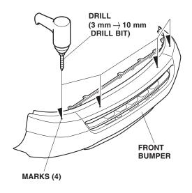
5. While wearing eye protecion, drill a 3 mm hole through each of the four dimples on the ends of the front bumper. Remove any burrs from the edges of the holes with a file.
