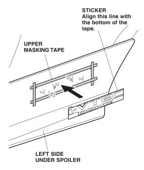
43. While holding the "i-VTEC DOHC" sticker to keep it from moving, work out the air bubbles with a squeegee.
