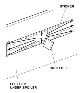
46. Remove the protective film from the outside of the "i-VTEC DOHC" sticker.
