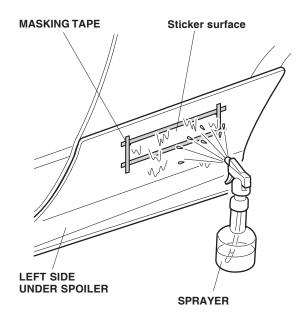
41. Fold back one end of the backing of the "i-VTEC DOHC" sticker, then spray the neutral detergent solution on the adhesive surface of the sticker.
