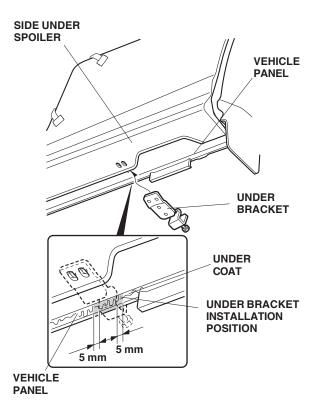
25. Cut into the marked area of the undercoat with a utility knife, and file off the undercoat from both sides of the vehicle panel.
