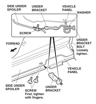
Position the under bracket on the side under spoiler and loosely install the two screws. Tighten the under bracket bolt, but don't tighten it completely yet. 31. Align the rear top edge of the left side under spoiler with the edge of the radius of the vehicle panel as shown. Remove the five adhesive tapes from the left side under spoiler. Press firmly on the side under spoiler firmly.
