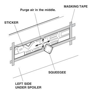
44. Spray the dish soap solution onto the protective film of the "i-VTEC DOHC" sticker. Remove the masking tapes.
