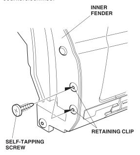
20. Using a self-tapping screw, pierce a hole through the center of the inner fender retaining clips.
