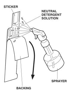
42. Align the upper edge of the "i-V-TEC DOHC" sticker with the bottom of the upper masking tape, and attach it to the side under spoiler.
