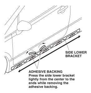
When the workshop room temperature is below 60°F(15°C), warm up the entire side lower bracket to 60°F(15°C) or above before attaching it to the vehicle body.
