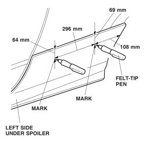
38. Attach masking tapes on the left side under spoiler as illustrated.
