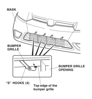
17. Attach the four plastic hooks to the bottom inside edge of the bumper grille opening.
