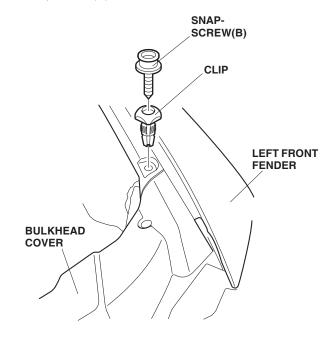
4. Repeat steps 2 and 3 to install a snap-screw(B) on the right side of the vehicle.
