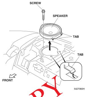
8. Install the right and left speakers using the screws removed in step 7.
