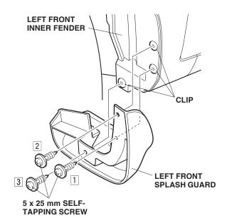
Turn the steering wheel all the way clockwise, and repeat steps 2 and 3 to install the right front splash guard.
