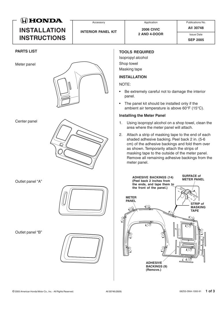
3. Position the meter panel on the existing meter panel. While holding pressure on the meter panel, carefully remove the adhesive backings from the meter panel. Hold the meter panel firmly against the existing meter panel with the palm of your hand, particularly at the edges.
