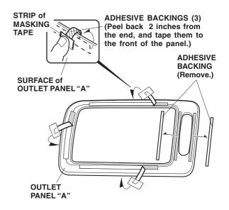
8. Attach a strip of masking tape to the end of each shaded adhesive backing. Peel back 2 in. (5-6 cm) of the adhesive backings and fold them over as shown. Temporarily attach the strips of masking tape to the outside of outlet panel "A". Remove all remaining adhesive backings from outlet panel "A".
