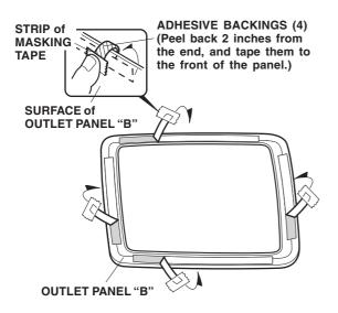
10. Position the outlet panels "A" and "B" on the existing outlet panels. While holding pressure on the outlet panels, carefully remove the adhesive backings from the outlet panels. Hold the outlet panels "A" and "B" firmly against the existing outlet panels with the palm of your hand, particularly at the edges.
