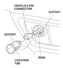
Align the locating tab on the socket with the cutout in the ring, and slide the socket into the ring. 10. Push the cigarette lighter into the socket.
