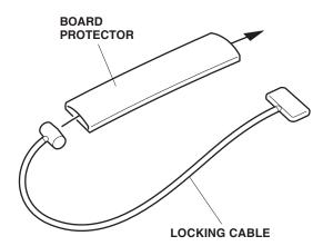
14. Insert the locking cable plate into the slot of the snowboard carrier. To carry one snowboard, insert the plate into the lowest slot. To carry two snowboards, use one of the three upper slots in the carrier.
