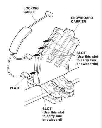
15. After loading each snowboard on the carrier, adjust it with the help of the board supports so that the top edges are level and the boards are as far down in the carrier as possible. To secure the snowboard use the key to open the covers, then insert the locking cable stoppers into the holes of the carrier covers.
