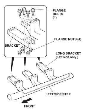
2. Position the left side step on the body, and loosely install the twelve flange bolts.
