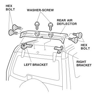
Tighten the four hex bolts and the two washerscrews. 10. Install the two bolt covers on the rear air deflector. Position the cover toward the rear of the opening when installing.
