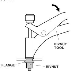
(4) Release the handle, turn the mandrel, and remove it from the rivnut.
