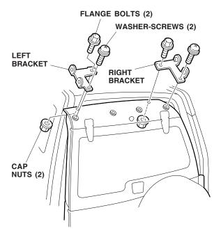
8. Position the rear air deflector on the brackets, and install two washer-screws and four hex bolts.
