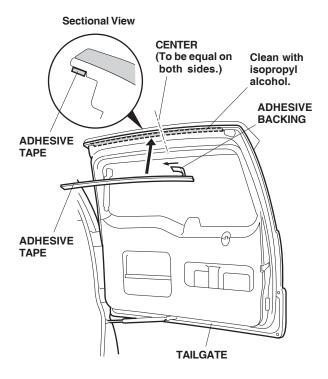
12. Attach the adhesive tape along the upper edge of the tailgate.
