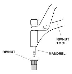
(2) Insert the rivnut into the hole in the body panel.
