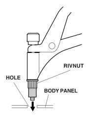
(3) Squeeze the handle firmly until the rivnut is compressed to form a flange-like stopper under the body panel.
