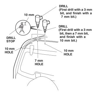
6. Install the rivnuts in the tailgate as described in substeps (1) through (4) on page 3.
